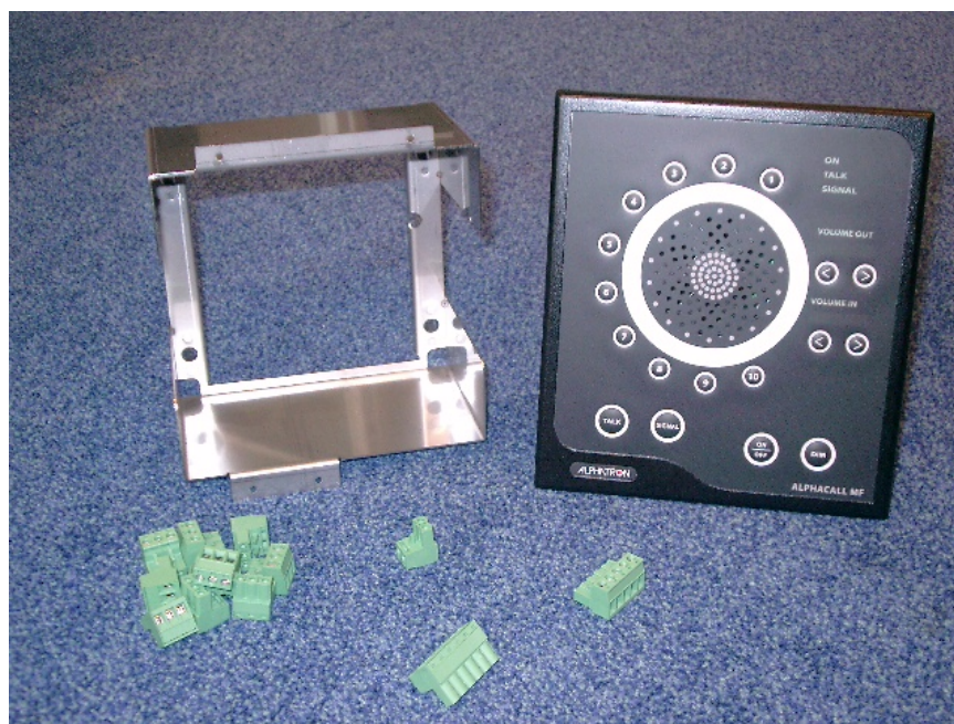
Figure 1: The complete hardware of the ALPHACALL MF
