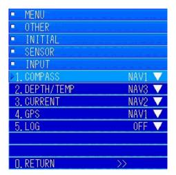
In the [SENSOR SETTINGS] menu, turn the [MULTI] knob to select "1. INPUT". Press the [MULTI] knob to display the submenu.
