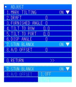
When such strong signals as propeller noise are input, it impacts surrounding images. The specialized function "STERN BLANK" is included for this reason. In the [6. ADJUST] menu, turn the [MULTI] knob to select "7. STERN BLANK". Press the [MULTI] knob to display the pulldown menu.
