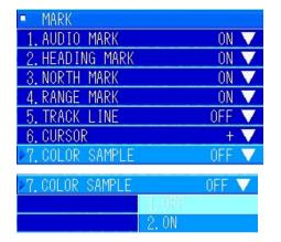
Turn the [MULTI] knob to select "7. COLOR SAMPLE". Press the [MULTI] knob to display the pulldown menu.
