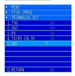
Move to the "TECHNOLOG SET" menu and turn the [MULTI] knob to move to "5. ADC". Press the [MULTI] knob to open the menu for entering values, and then do the settings for 0 through 7.
