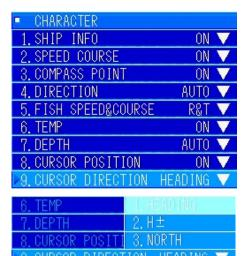
Turn the [MULTI] knob to select "9. CURSOR DIRECTION". Press the [MULTI] knob to display the pulldown menu.
