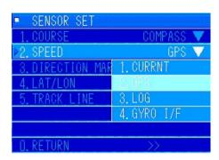
In the [SENSOR SET] menu, turn the [MULTI] knob to select "2. SPEED". Press the [MULTI] knob to display the pulldown menu.
