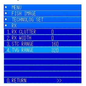
In the "RECEIVE" menu, turn the [MULTI] knob to move to [4. TVG RANGE]. Press the [MULTI] knob to display the menu for entering values.
