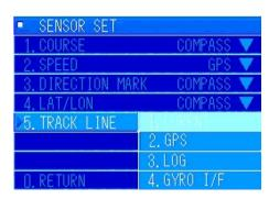
In the [SENSOR SET] menu, turn the [MULTI] knob to select "5. TRACK LINE". Press the [MULTI] knob to display the pulldown menu.
