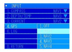
In the [INPUT] menu, turn the [MULTI] knob to select "4. GPS". Press the [MULTI] knob to display the pulldown menu.
