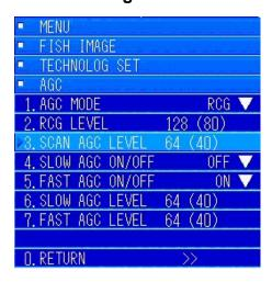
In the "AGC" menu, turn the [MULTI] knob to move to [3. SCAN AGC LEVEL]. Press the [MULTI] knob to display the menu for entering values.
