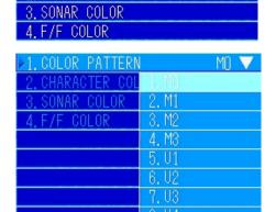
Turn the [MULTI] knob to select "1. COLOR PATTERN". Press the [MULTI] knob to display the pulldown menu.
