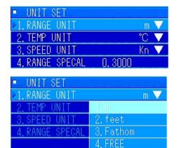
In the [7. UNIT SET] menu, turn the [MULTI] knob to select "1. RANGE UNIT". Press the [MULTI] knob to display the pulldown menu.
