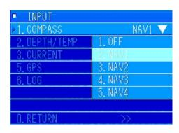
In the [INPUT] menu, turn the [MULTI] knob to select "1. COMPASS". Press the [MULTI] knob to display the pulldown menu.
