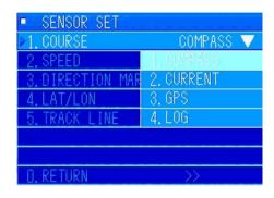
In the [SENSOR SET] menu, turn the [MULTI] knob to select "1. COURSE". Press the [MULTI] knob to display the pulldown menu.
