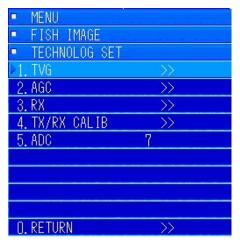
Move to the "TECHNOLOG SET" menu and turn the [MULTI] knob to move to "1.TVG". Press the [MULTI] knob to open the submenu.
