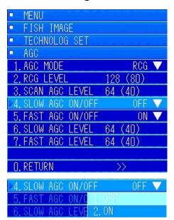
In the [AGC] menu, turn the [MULTI] knob to move to [4. SLOW AGC ON/OFF]. Press the [MULTI] knob to display the pulldown menu.
