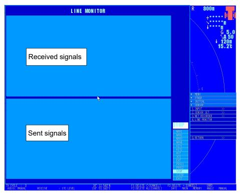
In the [SENSOR] menu, turn the [MULTI] knob to select "4. LINE MONITOR". Press the [MULTI] knob to display the specialized screen for the "LINE MONTOR".
