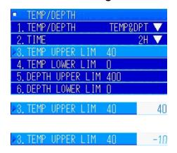
Turn the [MULTI] knob to select "3. TEMP UPPER LIM". Press the [MULTI] knob to display the menu for inputting values.
