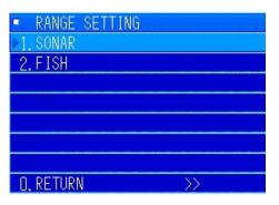
In the [3. RANGE SETTING] menu, turn the [MULTI] knob to select "1. SONAR". Press the [MULTI] knob to accept.
