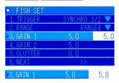
Turn the [MULTI] knob to select "3. GAIN 1". Press the [MULTI] knob to display the menu for inputting values. Turn the [MULTI] knob to adjust the image to be close to the image of the fish finder that is connected.
