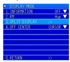
Turn the [MULTI] key to select "3. SPLIT DISPLAY". Press the [MULTI] knob to display the submenu, select either "1. AUDIO" or "2. F/F", and then set it.
