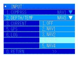
In the [INPUT] menu, turn the [MULTI] knob to select "2. DEPTH/TEMP". Press the [MULTI] knob to display the pulldown menu.
