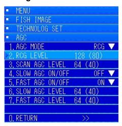
In the "AGC" menu, turn the [MULTI] knob to move to [2. RCG LEVEL]. Press the [MULTI] knob to display the menu for entering values.
