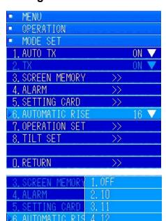
Press the [MENU] key to display the menus. Turn the [MULTI] knob to select "8. MODE SET". Press the [MULTI] knob to open the submenu.
