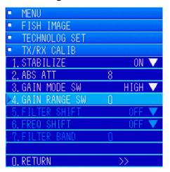
In the "TX/RX CALIB" menu, turn the [MULTI] knob to move to [4. GAIN RANGE SW]. Press the [MULTI] knob to display the menu for entering values.
