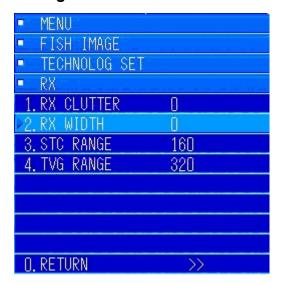
In the "RECEIVE" menu, turn the [MULTI] knob to move to [3. RX WIDTH]. Press the [MULTI] knob to display the menu for entering values.
