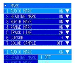
Turn the [MULTI] knob to select "1. AUDIO MARK". Press the [MULTI] knob to display the pulldown menu.
