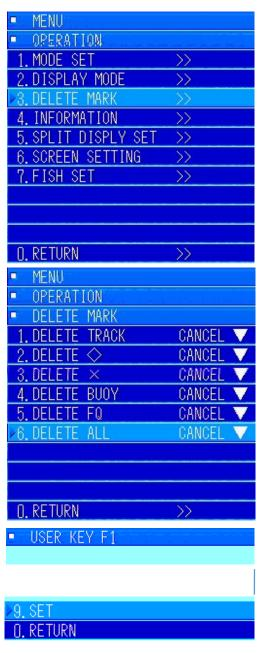
The procedure for registering "DELETE ALL" to the [F1] key is explained as an example.
