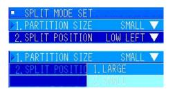
Turn the [MULTI] knob to select "1. PARTITION SIZE". Press the [MULTI] knob to display the pulldown menu.
