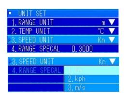
In the [7. UNIT SET] menu, turn the [MULTI] knob to select "3. SPEED UNIT". Press the [MULTI] knob to display the pulldown menu.
