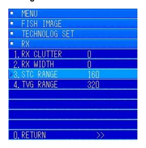
In the "RECEIVE" menu, turn the [MULTI] knob to move to [4. STC RANGE]. Press the [MULTI] knob to display the menu for entering values.
