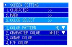
Follow the menu operations for screen settings to display the "SCREEN SETTING" submenu.
