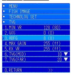
In the "TVG" menu, turn the [MULTI] knob to move to [3. ABFG]. Press the [MULTI] knob to open the value input key menu.
