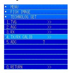
Move to the "TECHNOLOG SET" menu and turn the [MULTI] knob to move to "4. TX/RX CALIB". Press the [MULTI] knob to open the submenu.
