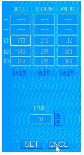
After doing the color settings, align the cursor with "SET" and press the [ENT] key to complete the settings.
