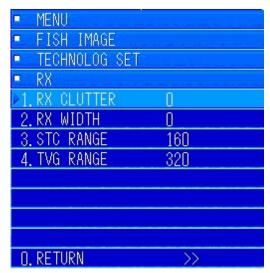
Move to the "TECHNOLOG SET" menu and turn the [MULTI] knob to move to "3. RX". Press the [MULTI] knob to open the submenu.
