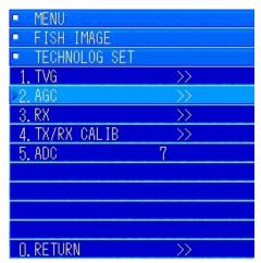
Move to the "TECHNOLOG SET" menu and turn the [MULTI] knob to move to "2. AGC". Press the [MULTI] knob to open the submenu.
