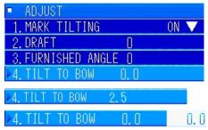
In the [6. ADJUST] menu, turn the [MULTI] knob to select "4. TILT TO BOW ". Press the [MULTI] knob to display the menu for inputting values.
