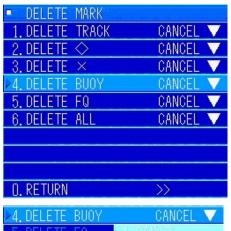
Follow the operations for deleting marks. Open the "DELETE MARK" menu. Turn the [MULTI] knob to select "4. DELETE BUOY". Press the [MULTI] knob to display the pulldown menu.
