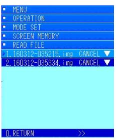
While the recorded screen data is being written, the name of the file that is being written is displayed as shown in the diagram on the left.
