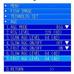
In the "AGC" menu, turn the [MULTI] knob to move to [7. FAST AGC LEVEL]. Press the [MULTI] knob to display the menu for entering values.
