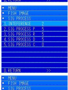
Turn the [MULTI] knob to move to "1. INTEFERENCE". Press the [MULTI] knob to open the menu for entering values.
