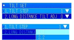
Turn the [MULTI] knob to select "1. TILT STEP". Press the [MULTI] knob to open the pulldown menu.
