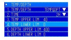
Turn the [MULTI] knob to select "4. TEMP LOWER LIM". Press the [MULTI] knob to display the menu for inputting values.
