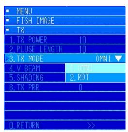
In the example on the left, selecting "3. TX MODE" with the [3] key or the [MULTI] knob opens the pull down menu. The number of menus varies depending on the item.
