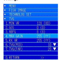
In the "TVG" menu, turn the [MULTI] knob to move to "4. MAX GAIN". Press the [MULTI] knob to open the value input key menu.
