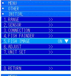
Open the "1. INITIAL" menu. Turn the [MULTI] knob to move to "5. FISH IMAGE", and then press the [MULTI] knob to open the pulldown menu.
