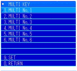
Turn the [MULTI] knob to move to "1. MULTI No.1" and press the [MULTI] knob to set "1. CLUTTER". (Registration is not yet complete)
