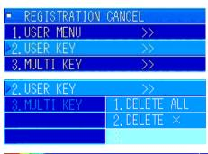
Open the "3. REGISTRATION CANCEL" menu. Turn the [MULTI] knob to move to "2. USER KEY". Press the [MULTI] knob to open the pulldown menu.
