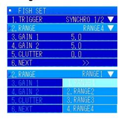
Turn the [MULTI] knob to select "2. RANGE". Press the [MULTI] knob to display the pulldown menu.
