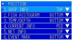
Press the [MULTI] knob to open the submenu. You can set the positions of items 1 through 6.
