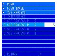
Turn the [MULTI] knob to move to "3. SIG PROCESS R". Press the [MULTI] knob to open the menu for entering values.
