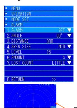
To turn the alarm function "On", turn the [MULTI] knob to move to "1. ALARM". Press the [MULTI] knob to display the pulldown menu, as shown in the diagram below.
