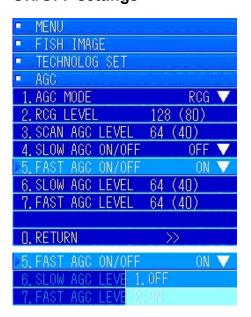
In the [AGC] menu, turn the [MULTI] knob to move to [5. FAST AGC ON/OFF]. Press the [MULTI] knob to display the pulldown menu.
