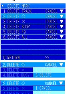
Follow the operations for deleting marks. Open the "DELETE MARK" menu. Turn the [MULTI] knob to select "2. DELETE  $\diamondsuit$ ". Press the [MULTI] knob to display the pulldown menu.
