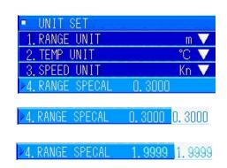
In the [7. UNIT SET] menu, turn the [MULTI] knob to select "4. RANGE SPECAL". Press the [MULTI] knob to display the menu for inputting values.
