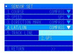
In the [SENSOR SET] menu, turn the [MULTI] knob to select "4. LAT/LON". Press the [MULTI] knob to display the pulldown menu.
