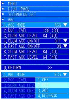
In the [AGC] menu, turn the [MULTI] knob to move to [1. AGC MODE]. Press the [MULTI] knob to display the pulldown menu.
