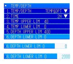
Turn the [MULTI] knob to select "6. DEPTH LOWER LIM". Press the [MULTI] knob to display the menu for inputting values.
