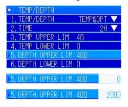
Turn the [MULTI] knob to select "5. DEPTH UPPER LIM". Press the [MULTI] knob to display the menu for inputting values.
