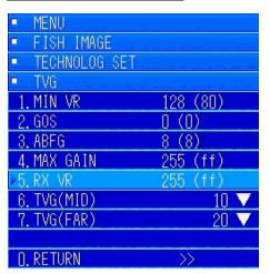
In the "TVG" menu, turn the [MULTI] knob to move to "5. RX VR". Press the [MULTI] knob to open the value input key menu.
