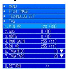
In the "TVG" menu, turn the [MULTI] knob to move to "1. MIN VR". Press the [MULTI] knob to open the value input key menu.
