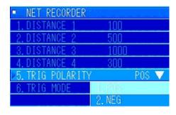
In the [NET RECORDER] menu, turn the [MULTI] knob to select "5. TRIG POLARITY". Press the [MULTI] knob to display the pulldown menu.
