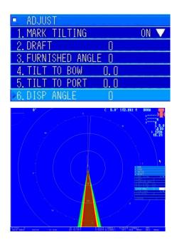
In the [6. ADJUST] menu, turn the [MULTI] knob to select "6. DISP ANGLE". Press the [MULTI] knob to display the menu for inputting values.
