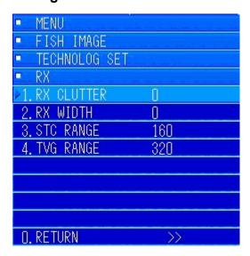
In the "RECEIVE" menu, turn the [MULTI] knob to move to [2. RX CLUTTER]. Press the [MULTI] knob to display the menu for entering values.
