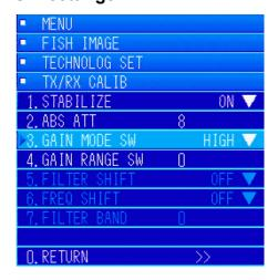
In the [TX/RX CALIB] menu, turn the [MULTI] knob to move to [1. STABILIZE]. Press the [MULTI] knob to display the pulldown menu.
