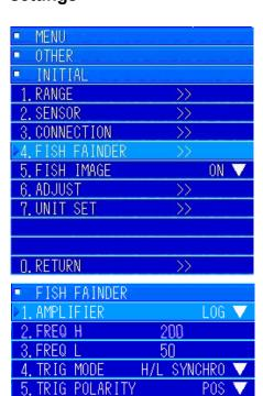
Open the "1. INITIAL" menu. Turn the [MULTI] knob to move to "4. FISH FINDER", and then press the [MULTI] knob to open the submenu.
