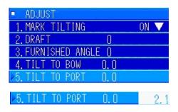
In the [6. ADJUST] menu, turn the [MULTI] knob to select "5. TILT TO PORT". Press the [MULTI] knob to show the display for inputting values.
