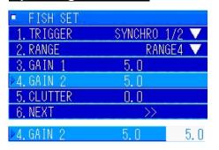
Turn the [MULTI] knob to select "4. GAIN 2". Press the [MULTI] knob to display the menu for inputting values. Turn the [MULTI] knob to adjust the image to be close to the image of the fish finder that is connected.
