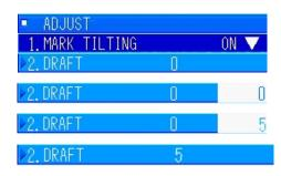
In the [6. ADJUST] menu, turn the [MULTI] knob to select "2. DRAFT". Press the [MULTI] knob to display the menu for inputting values.
