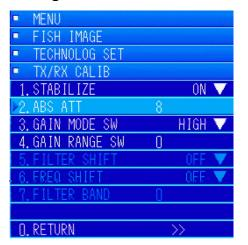
In the "TX/RX CALIB" menu, turn the [MULTI] knob to move to [2. ABS ATT]. Press the [MULTI] knob to display the menu for entering values.
