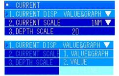
Turn the [MULTI] knob to select "1. CURRENT DISP". Press the [MULTI] knob to display the pulldown menu.
