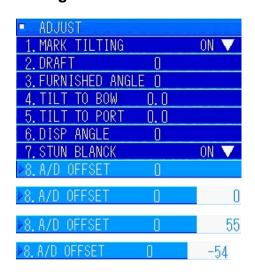
In the [6. ADJUST] menu, turn the [MULTI] knob to select "8. A/D OFFSET". Press the [MULTI] knob to display the menu for inputting values.
