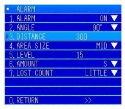
Use the [MULTI] knob to open the submenu for "ALARM" to do "ALARM" operations.
