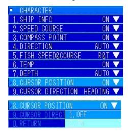
Turn the [MULTI] knob to select "8. CURSOR POSITION". Press the [MULTI] knob to display the pulldown menu.
