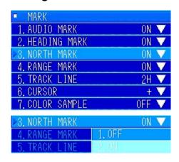
Turn the [MULTI] knob to select "3. NORTH MARK". Press the [MULTI] knob to display the pulldown menu.
