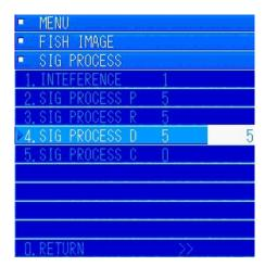
Turn the [MULTI] knob to move to "4. SIG PROCESS D". Press the [MULTI] knob to open the menu for entering values.
