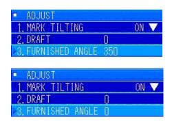
For the values to be input, you can set the heading as 0° and set the angle clockwise from 0° to 359° in steps of 1°. If the hoisting device is furnished in a direction that deviates 5° from the heading, set this setting to 355°. As an operation turn the [MULTI] knob counterclockwise and set to 355. Press the [MULTI] knob to assign it.
