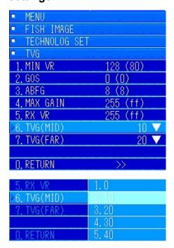
In the [TVG] menu, turn the [MULTI] knob to move to [6. TVG(MID)]. Press the [MULTI] knob to display the pulldown menu.
