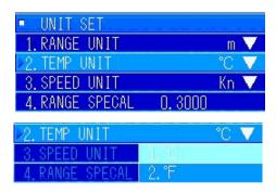
In the [7. UNIT SET] menu, turn the [MULTI] knob to select "2. TEMP UNIT". Press the [MULTI] knob to display the pulldown menu.
