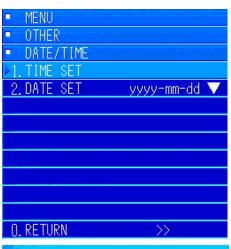
Move to "DATE/TIME". Press the [MULTI] knob to open the submenu. Turn the [MULTI] knob to move to "1. TIME SET" and a specialized menu opens.
