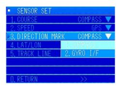
In the [SENSOR SET] menu, turn the [MULTI] knob to select "3. DIRECTION MARK". Press the [MULTI] knob to display the pulldown menu.
